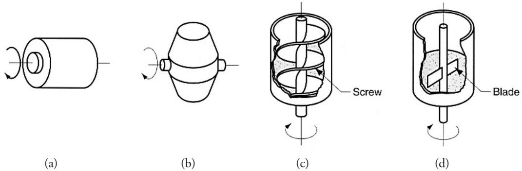
Several blending and mixing devices: (a) rotating drum, (b) rotating double cone, (c) screw mixer, (d) blade mixer
