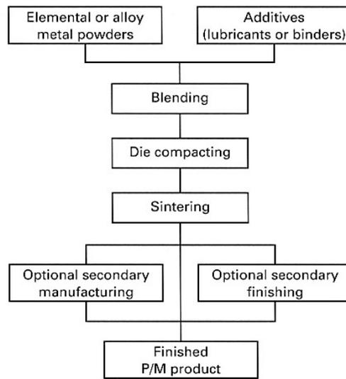
Simplified flowchart illustrating the sequence of operations in powder metallurgy process
