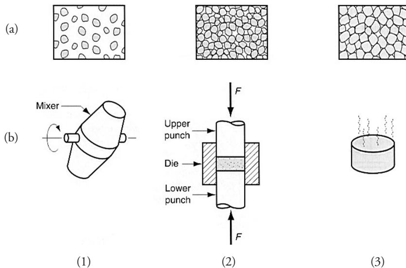
The conventional P/M process sequence: (1) blending, (2) compacting, and (3) sintering; (a) shows the condition of powders, and (b) shows the schematics of operation
