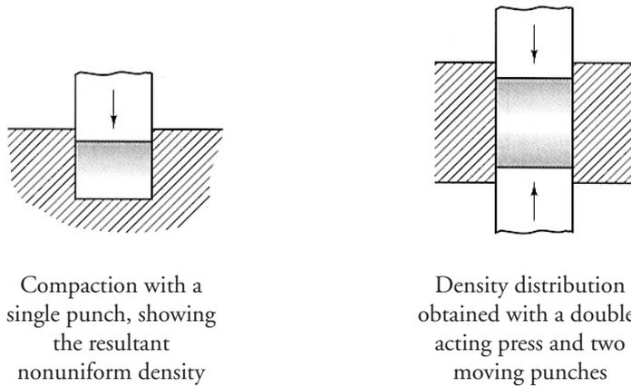
Compaction with a single punch, showing the resultant nonuniform density
