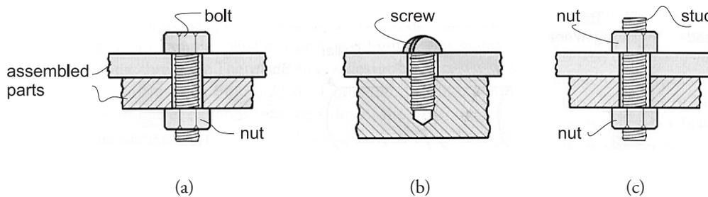
Typical assemblies using (a) bolt and nut, (b) screw and (c) stud and nut.
