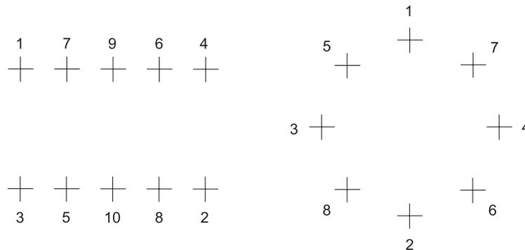
Sequence of tightening for multiple threaded joints.
