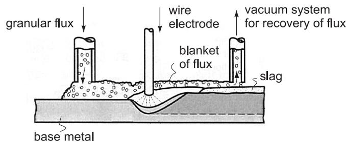
Submerged arc welding operation.
