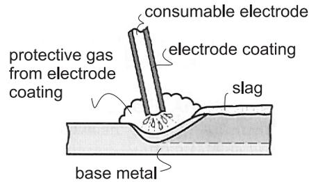
Shielded metal arc welding operation.
