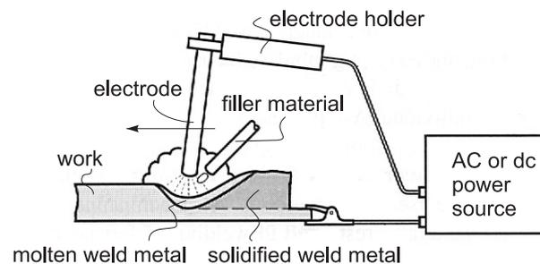
The basic configuration of an arc welding operation.
