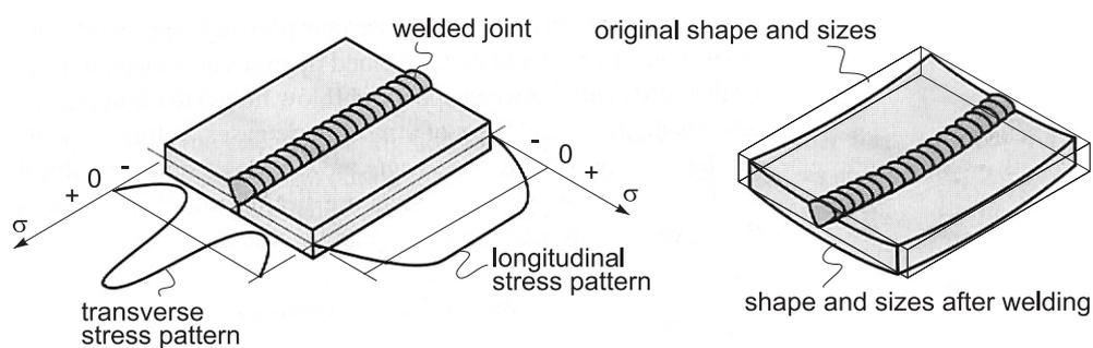
(Left) transverse and longitudinal residual stress pattern; and (Right) likely distortion in the welded assembly.
