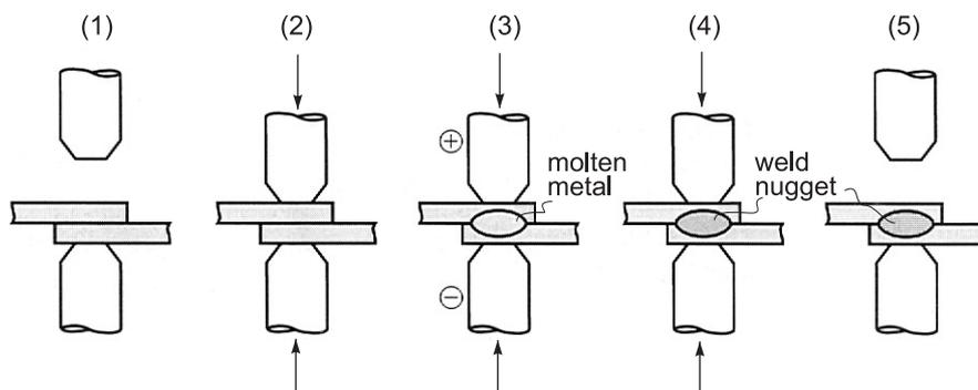
Steps in a spot welding cycle: (1) parts inserted between open electrodes, (2) electrodes close and force is applied, (3) weld time (current is switched), (4) current is turned off but force is maintained, and (5) electrodes are opened, and the welded assembly is removed.
