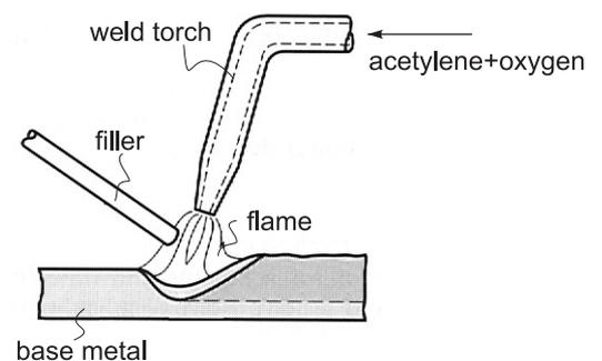
Oxyfuel gas welding operation.
