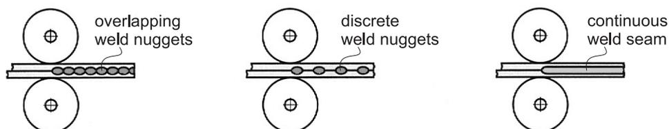
Different types of seam welding, (from left to right) conventional seam welding, roll spot welding, continuous resistance seam welding.
