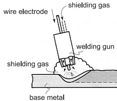
Gas metal arc welding operation.
