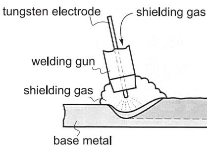
Gas tungsten arc welding operation.
