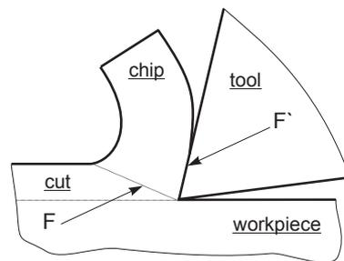
Total cutting force  $F$  and reaction force  $F'$  in orthogonal cutting
