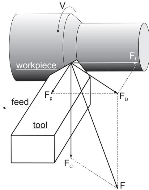
Force components in three-dimensional oblique cutting
