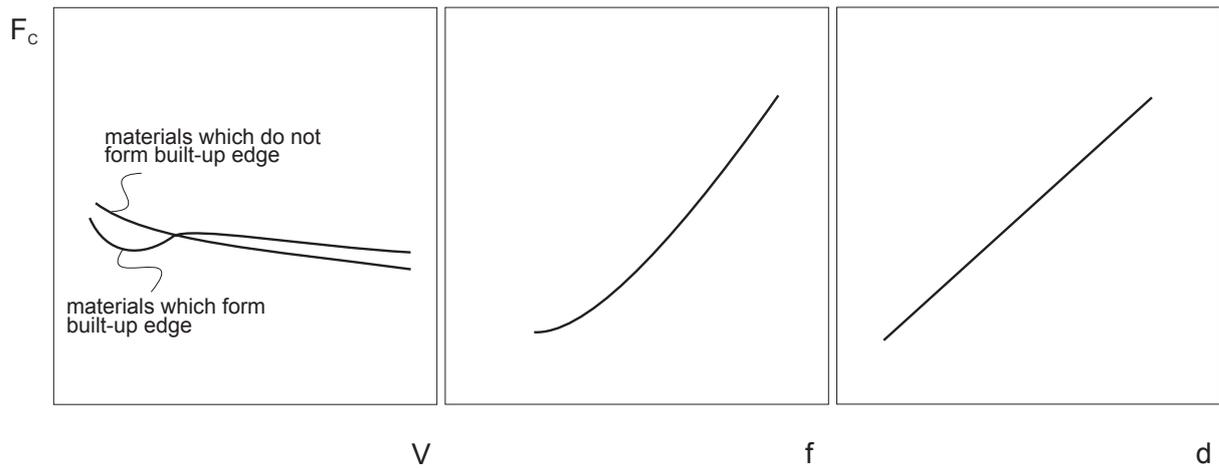
Cutting force as a function of cutting conditions
