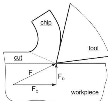
Total cutting force  $F$  is conveniently resolved into horizontal component  $F_C$  and vertical component  $F_D$
