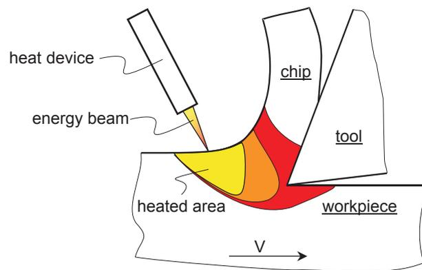
Oxyfuel torch used for thermally-assisted machining
