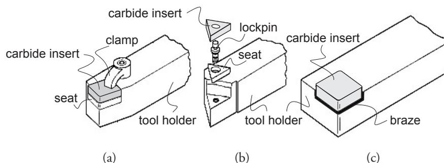
Methods of attaching carbide inserts to tool holder:
