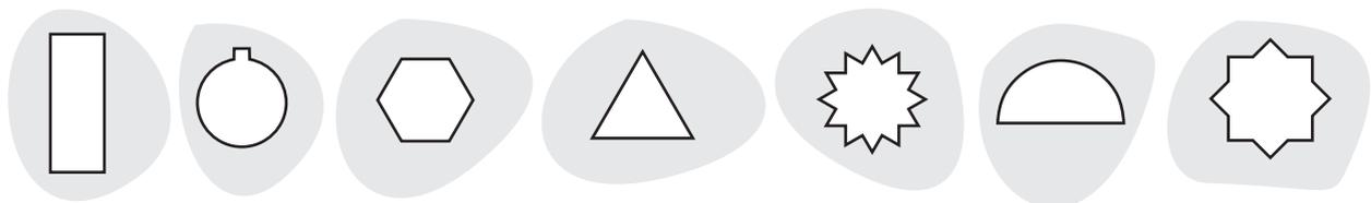
Various shapes produced by internal broaching operation.
