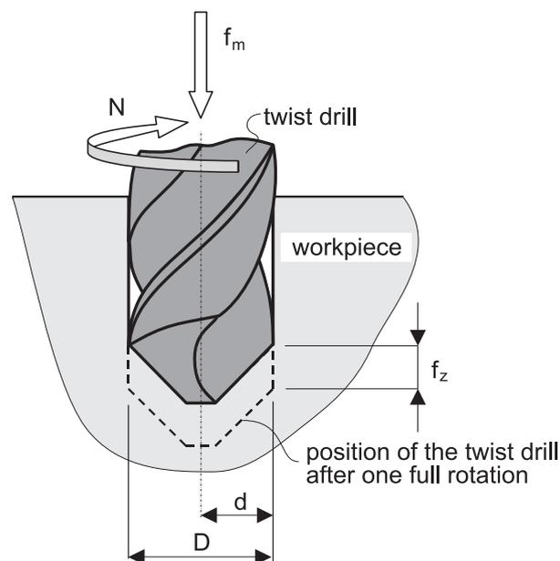
Basics of a drilling operation.
