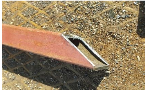
Figure 43 - Legs Cut at an Angle
