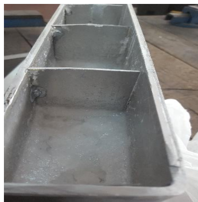
Figure 59 - Solidified PCM a Day Later
