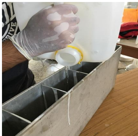
Figure 58 - Pouring PCM into Container
