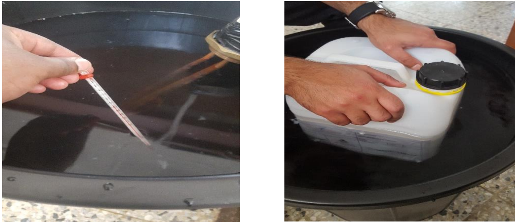
Figure 57 - Melting PCM Procedure
