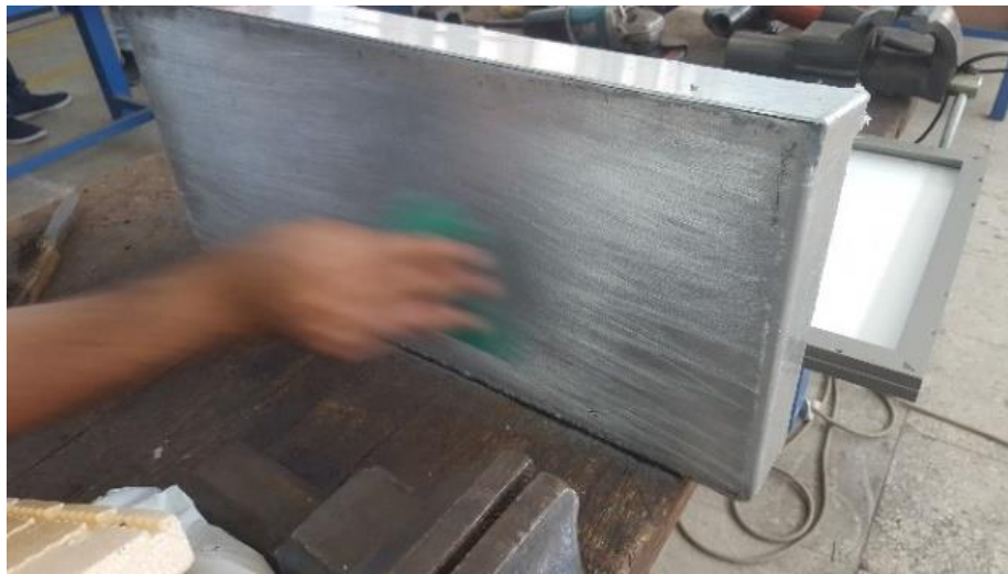
Figure 61 - Sanding of Container Surface
