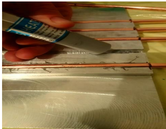
Figure 47 - Thermal Paste in HP Slots
