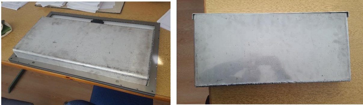
Figure 55 - PCM Container Post Welding
