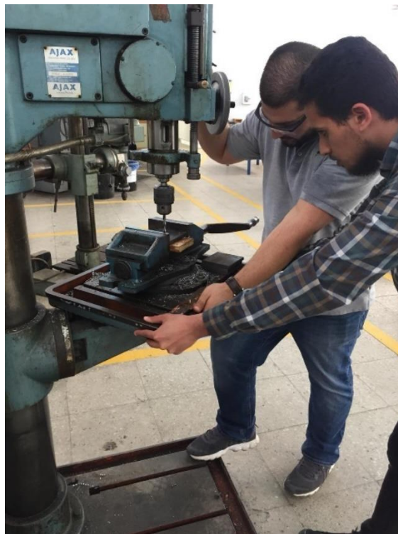
Figure 27: Drilling process for table wheels using a drill press machine.
