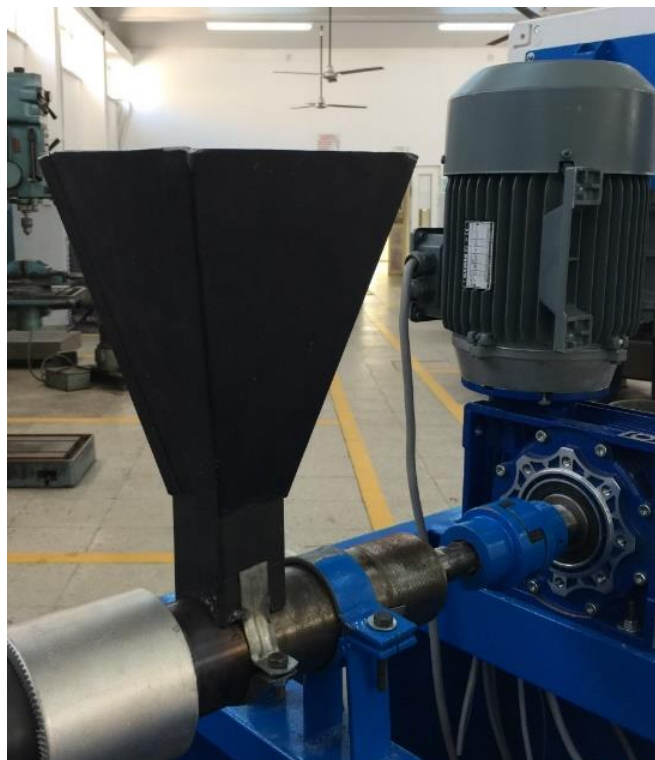
Figure 16: Selected hopper design.
