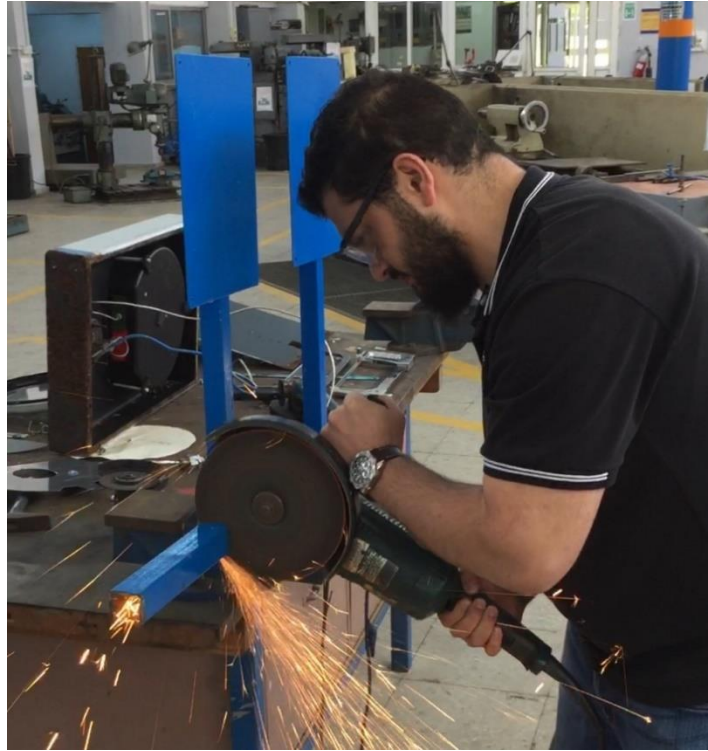
Figure 26: Cutting using portable abrasive cut-off machine.
