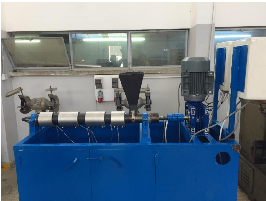
Figure 17: Plastic extrusion machine table. Note: complete table design configuration and dimensions are illustrated in Appendix J.
