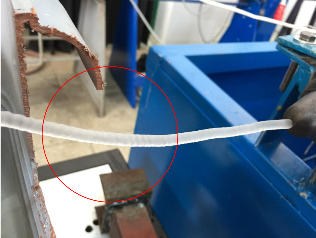
Figure 30: Extrudate profile (sharkskin defect) at low motor speed.
