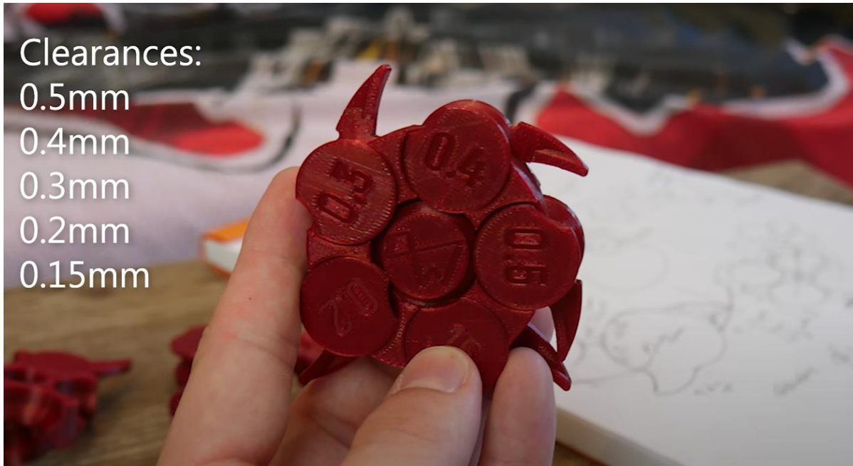
Figure 51: Clearance values of Tolerance Gauge Test part ("Clearance and Tolerance 3D Printer Gauge," n.d.)
