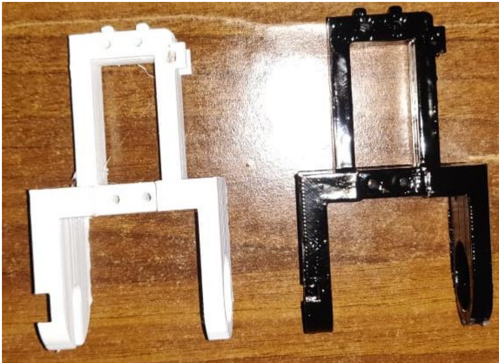
Figure 46 - Fresh printed 3D segment and sprayed segment.
