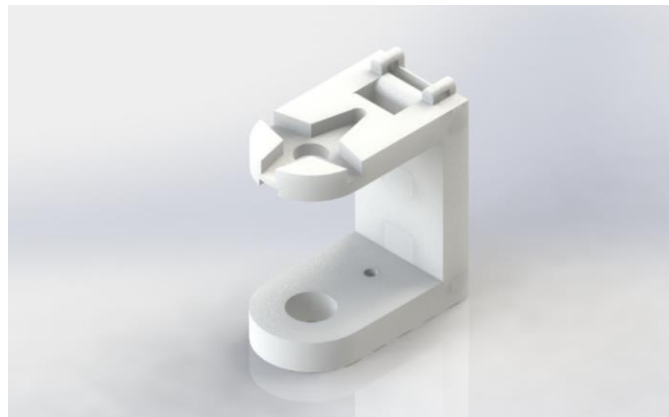
Figure 15: Nose servo mount design
