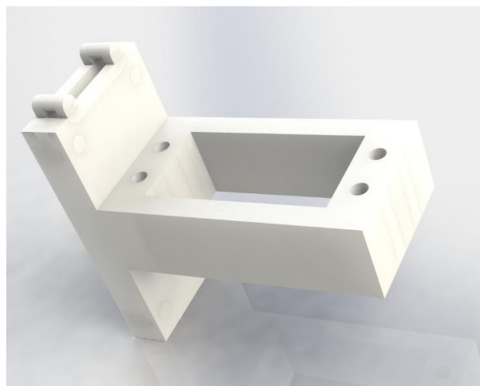
Figure 16: Tail servo mount design
