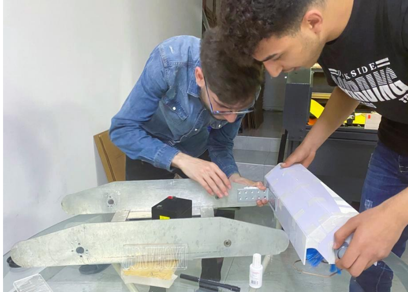
Figure 89. Pre-Alignment of Brush Mechanism with the Chassis
