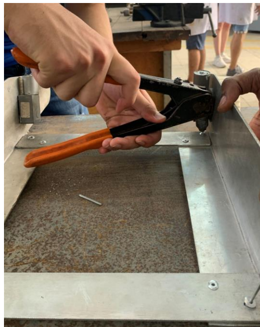
Figure 67. Riveting of Chassis
