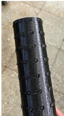
Figure 84. 3D Printed Brush Shaft
