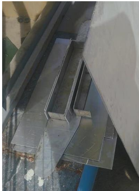
Figure 65. Chassis Parts from CNC and Bending Operations
