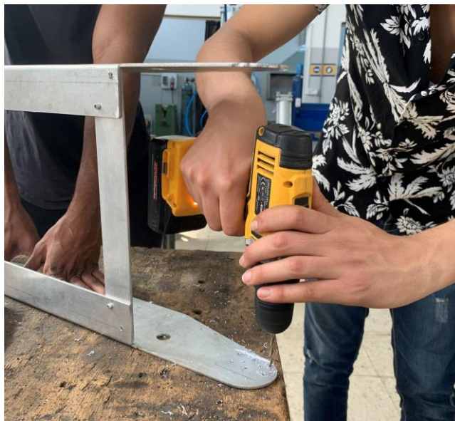
Figure 69. Drilling holes on the chassis
