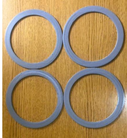
Figure 83. 3D Printed Wheel Rings
