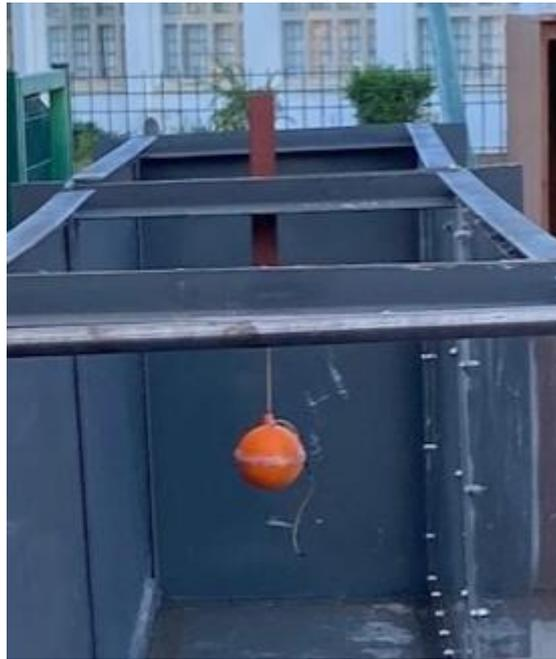
*Figure 47 Buoy attached to the wave tank third segment.*
