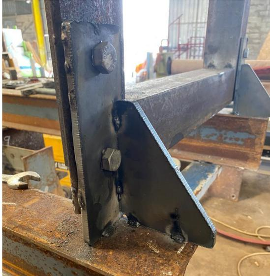
*Figure 39 Frame faces welded on two 6m I beams*
