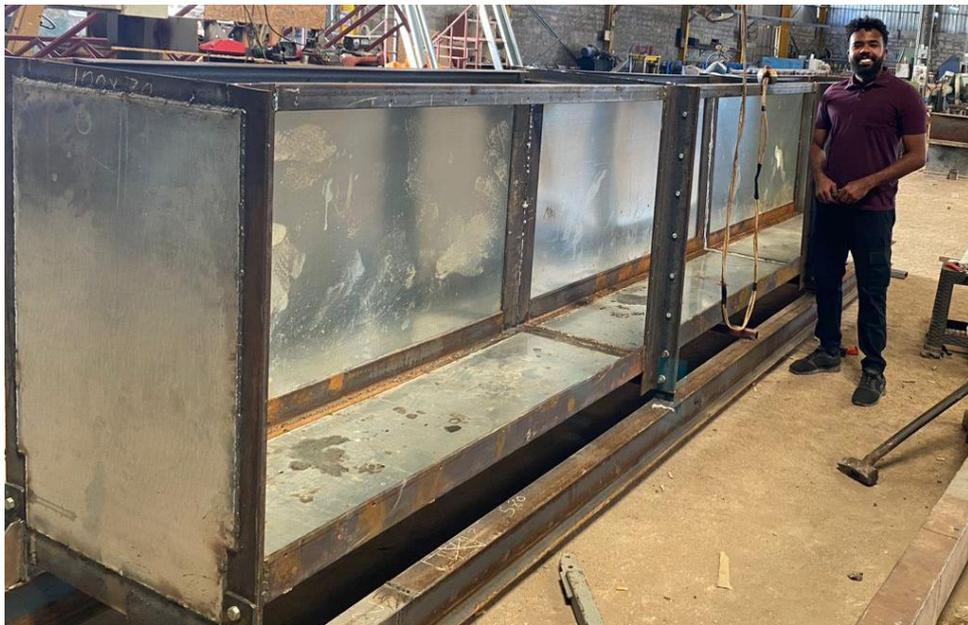
*Figure 43 Assembly of the 3 segments using bolts and washers*
