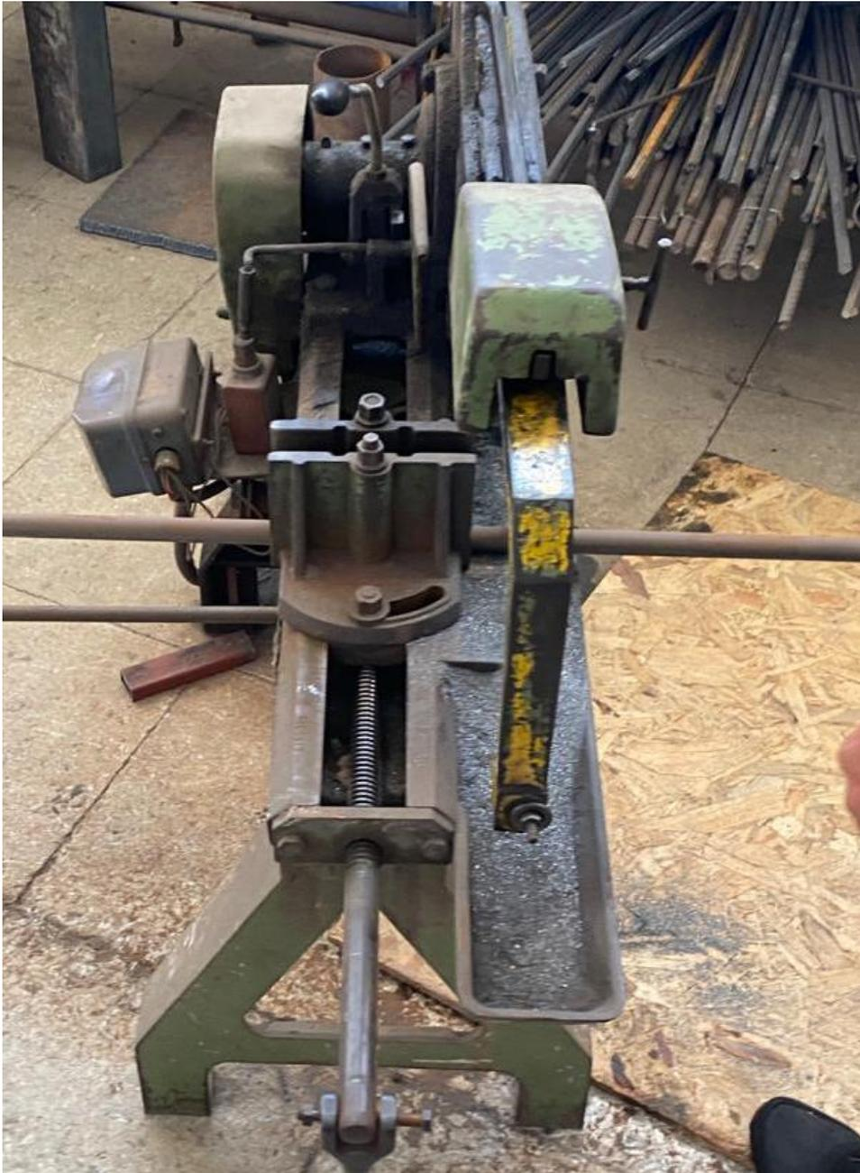
*Figure 44 Cutting the shaft with shearing machine*
