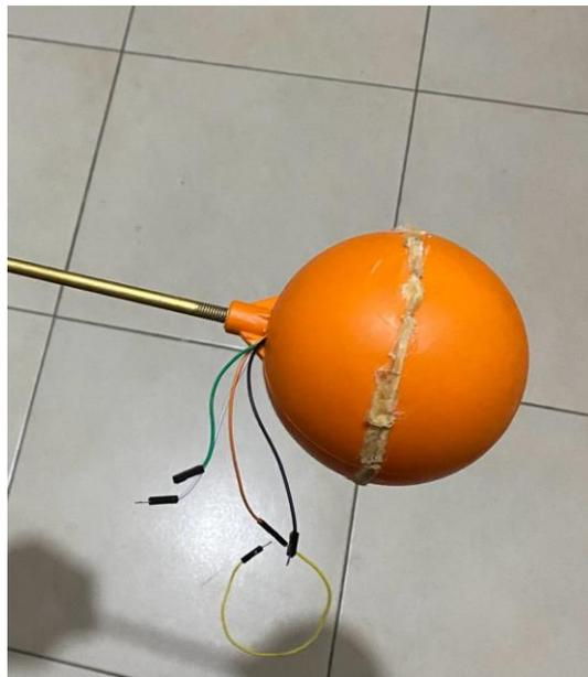
*Figure 46 Sensor buoy with accelerometer installed.*
