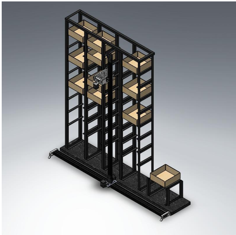
Figure 3.1-2 Design of the AS/RS
