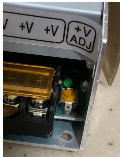
Figure 4.3-2 Voltage adjusting screw
