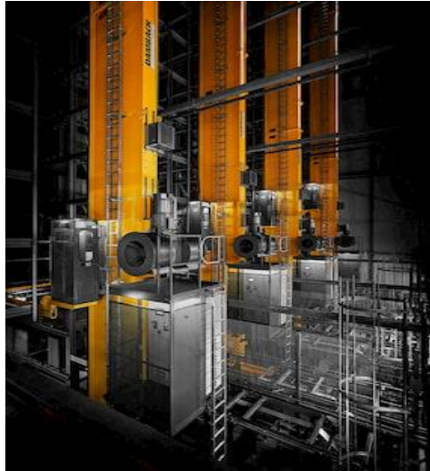
Figure 2.2-2 Fixed aisle AS/RS (Romaine, 2020)
