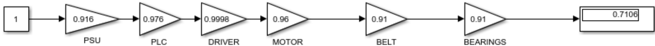
Figure 3.4-26 RBD with standby units
