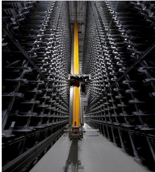
Figure 2.2-4 Mini-load AS/RS (Romaine, 2020)
