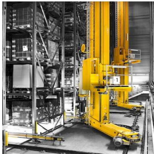
Figure 2.2-3 Movable aisle AS/RS (Romaine, 2020)
