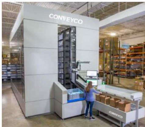
Figure 2.2-5 Shuttle based AS/RS (Romaine, 2020)
