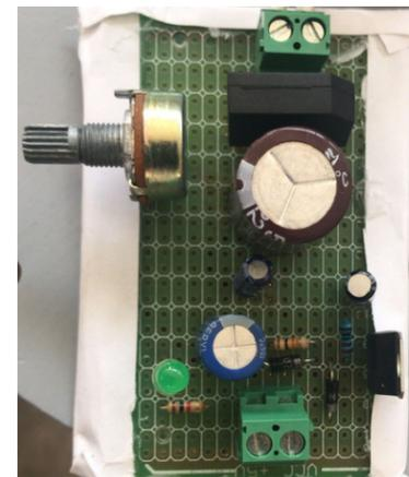
Rectifier circuit converts alternating current to direct current, and protects the battery from overload
