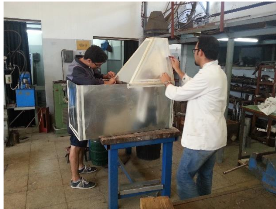
Figure 4.5 Applying Epoxy paste over welded part.
