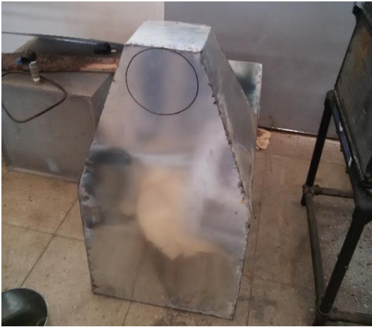
Figure E- 7 Manufacturing hole for the pipe.
