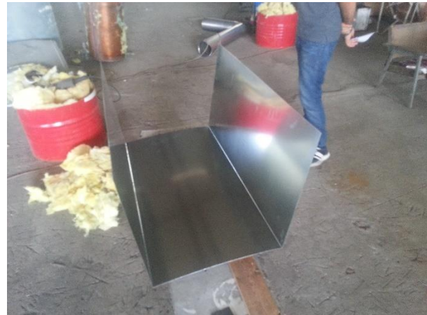
Figure E- 4 Manufacturing container base.
