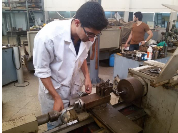
Figure E- 12 Modifying generator shaft 2.
