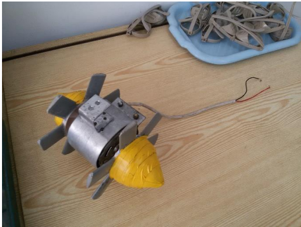
Figure E- 13 Turbine and generator assembly.
