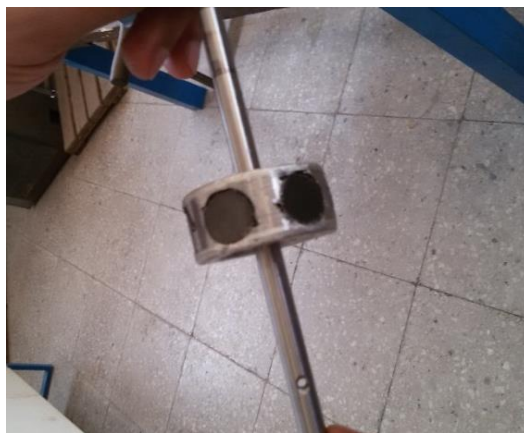
Figure 4.13 Fixing magnate on rotor.
