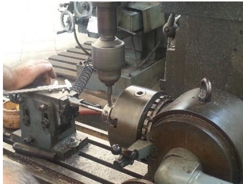
Figure 4.12 Drilling holes on external surface of the rotor.
