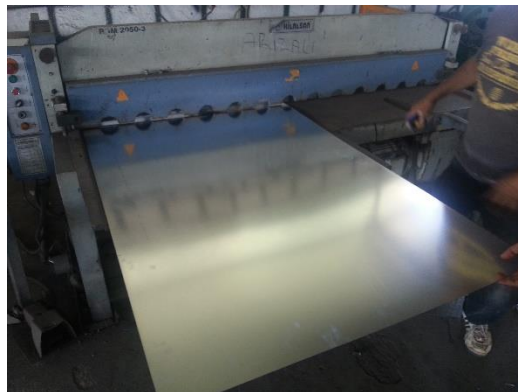
Figure 4.1 Cutting sheets metal by (Shearing-Machine).
