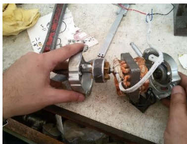
Figure 4.11 Disassemble fan motor.
