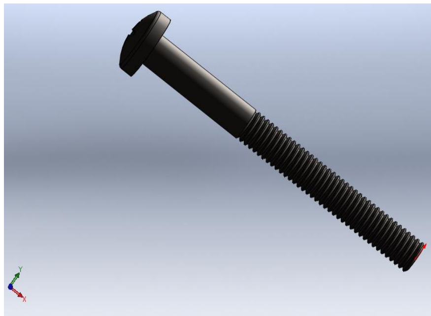
Figure 3. 8 : Screw M6 x 1.0 x 40 Type I Cross Recessed PHMS -38S
