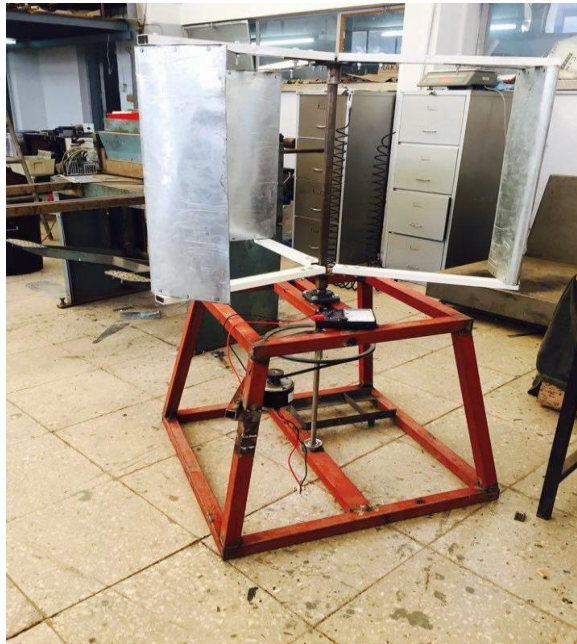
Figure 4. 8 : Final assembly of the Giromill wind turbine
