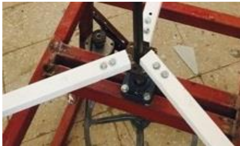
Figure 4. 5 : Arms final shape after manufacturing
