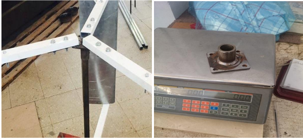
Figure 4. 6 : Radial arms fixing with supporters
