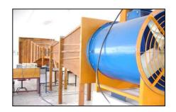
In the Aerodynamics Laboratory, there are two wind tunnels. Wind tunnels are used to study aerodynamics, effect of air, aerodynamic forces and how air flows through the tunnel. One of the wind tunnels has maximum capacity of 50 m/s with 10x40 cm test section and the other wind tunnel has the maximum capacity of 30 m/s with 50x50 test section.
