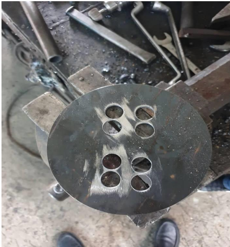
Figure 12 Drilled Tube Sheet
