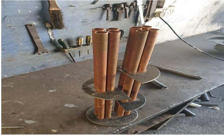
Figure 15 Copper tubes welded to both tube sheets and baffles
