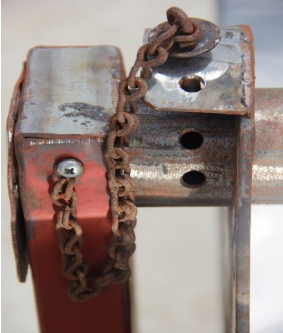
Figure 24. Mechanism to adjust the collector angle
