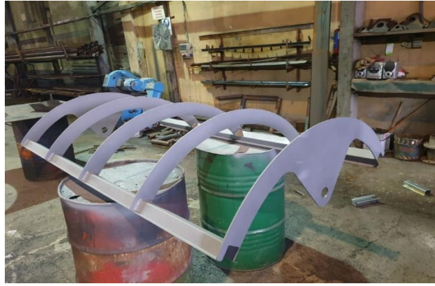
Figure 16. Ribs after assembling with channels
