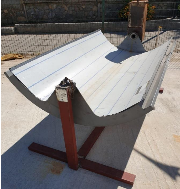
Figure 23. Collector after being attached to the frame
