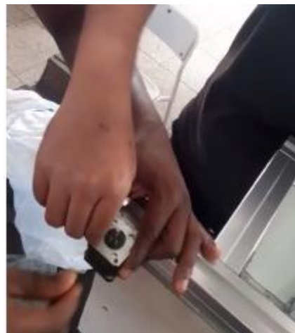
Figure 36: Fixing the bracket to the stepper motor.
