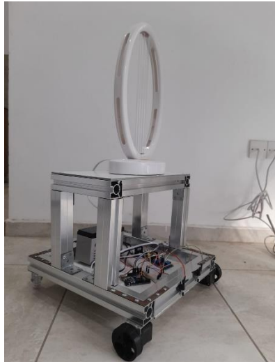
Figure 39: AGV with electronics (Side view)
