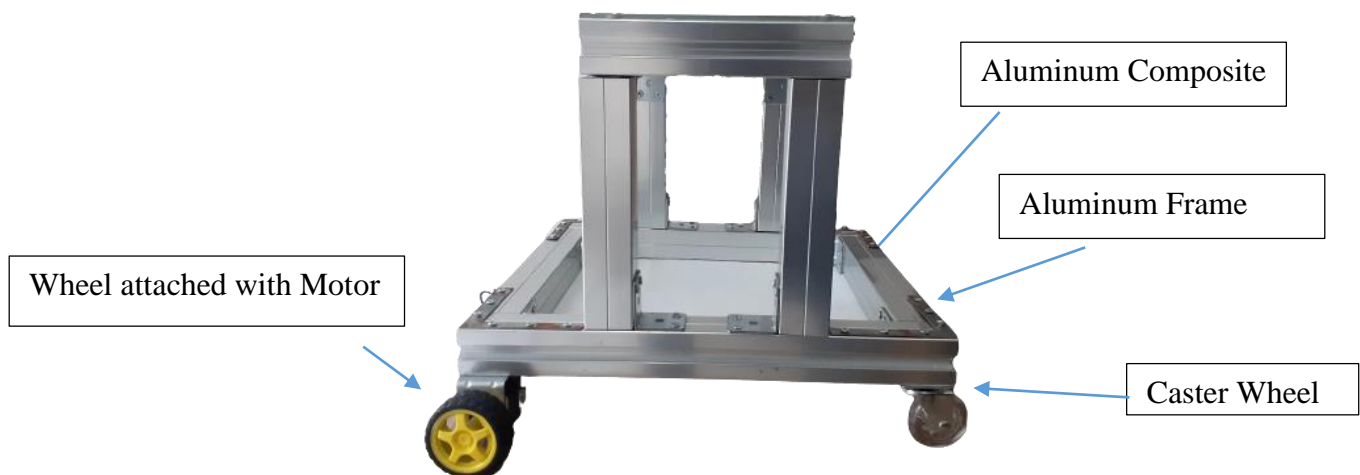
Figure 12: Labelled parts of AGV.
