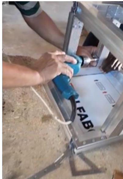
Figure 34: Screwing the four vertical frames to both the top and base.
