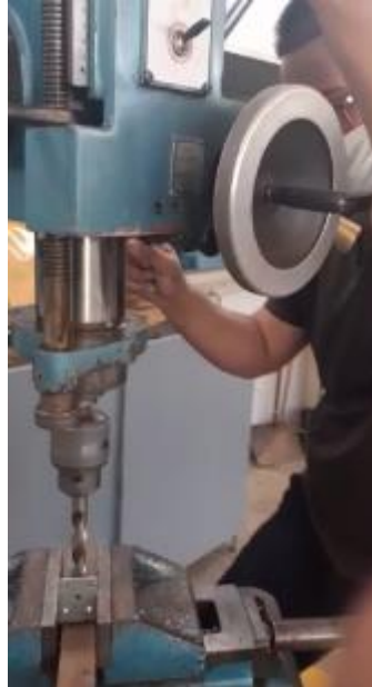
Figure 35: Drilling holes on a bracket to be used as stepper motor holder.
