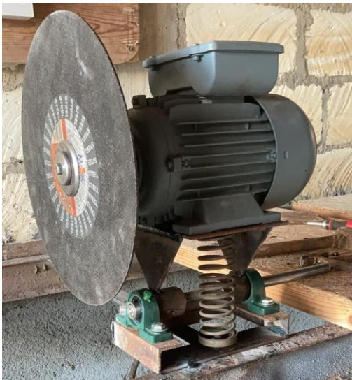
Figure 37 : Motor base & Support during manufacturing
