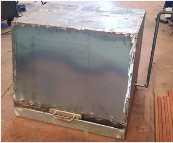
Figure 35 : Upper housing during manufacturing
