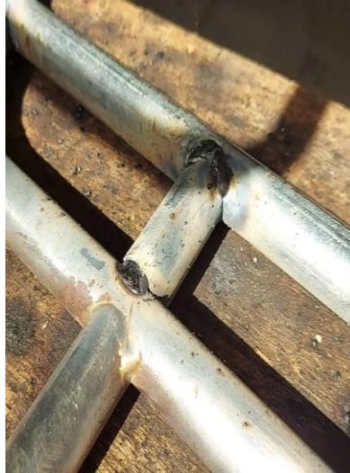
Figure 79: Caster tubes during welding
