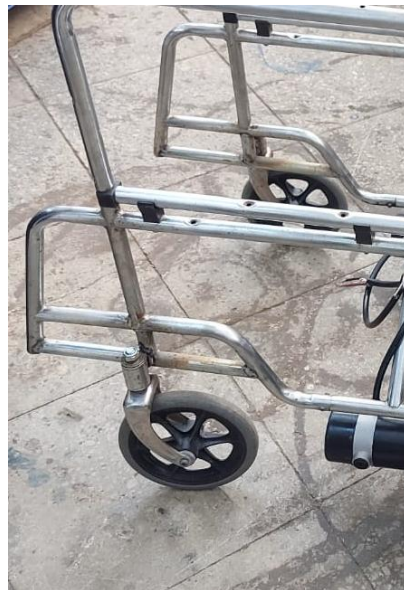
Figure 80: Caster before welding and after welding the new tube
