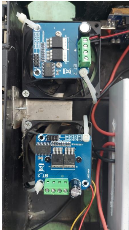
Figure 93: Motor drivers fixed in the Arduino box
