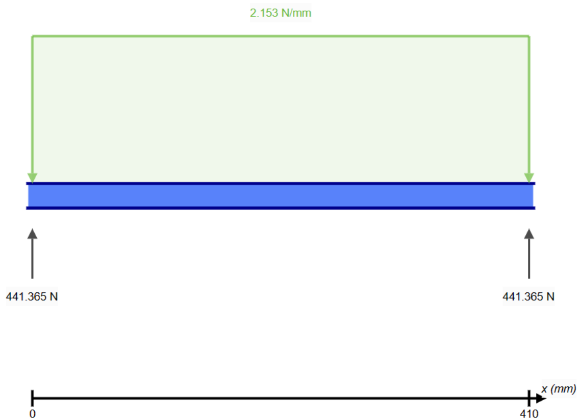
Figure 60: Freebody diagram of the wheelchair with assumptions
