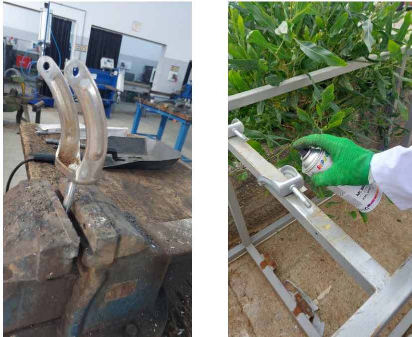
Figure 81: Caster fork before painting and after painting
