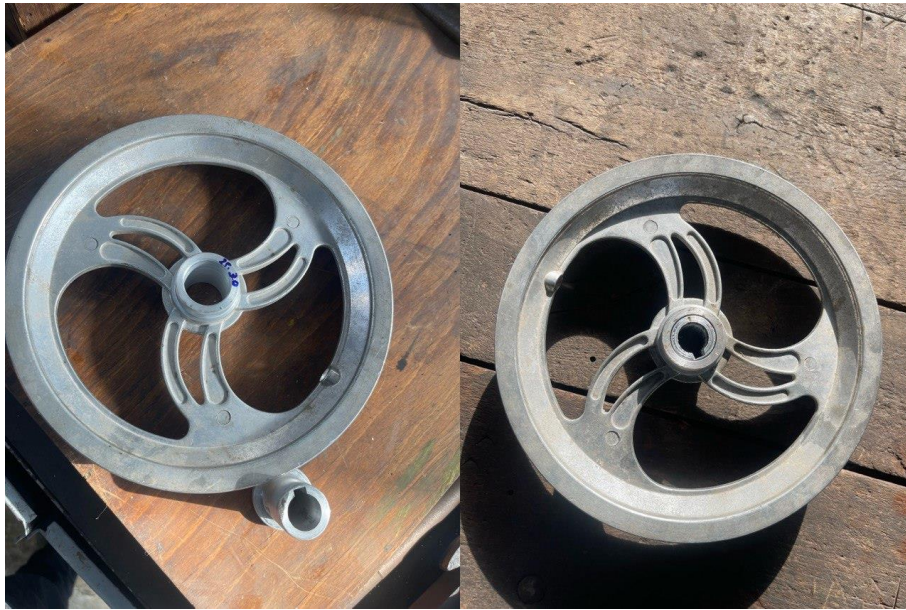
Figure 78: Machined connector fitted into wheels
