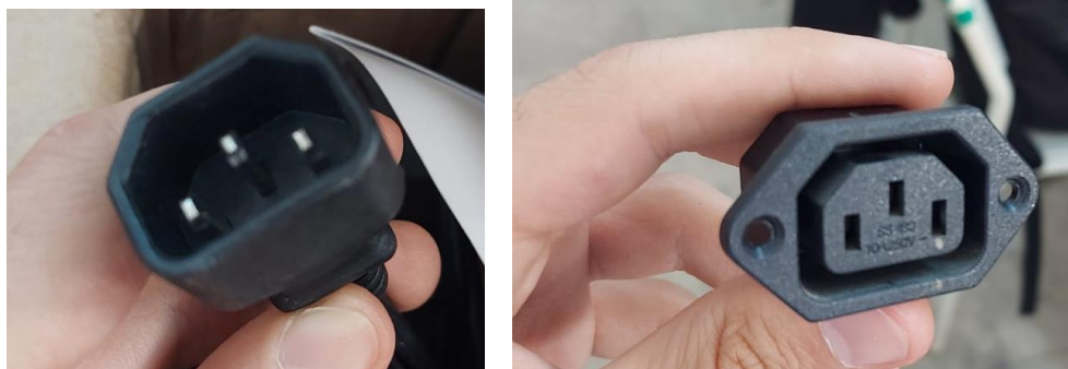
Figure 101: Connectors used for electrical connections between the battery and the Arduino box.
