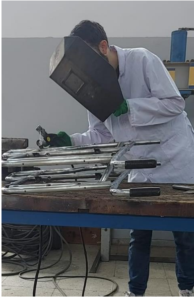
Figure 79: Caster tubes during welding
