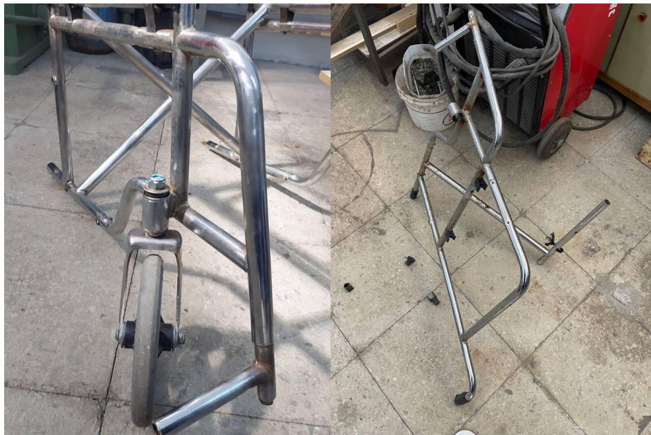
Figure 76: Dismantled frame before rust removal
